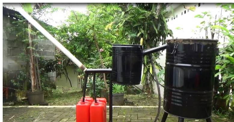
Figure 5. Installation of Liquid Smoke Production Equipment
