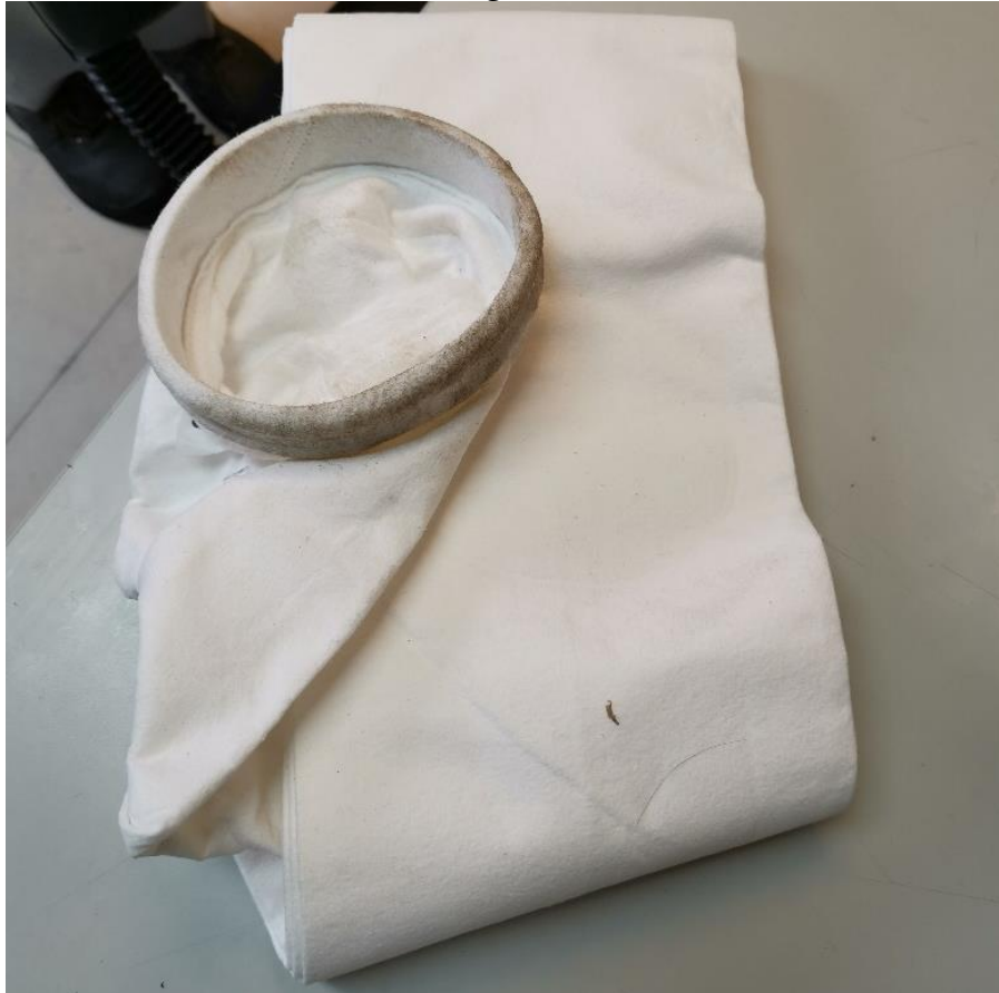
Figure 7. Filter Bag to Remove Dust (Image Source: Photographed by the Author)
