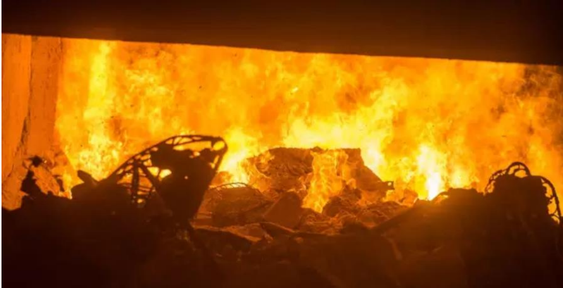
Figure 4. Garbage is Incinerated at Temperatures Above 850°C (Image Source: Government Information Bureau)
