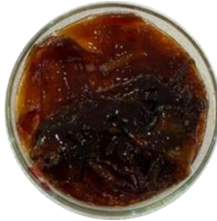
Figure 1. Liginosulfonate-Chitosan Hydrogel Fabrication
