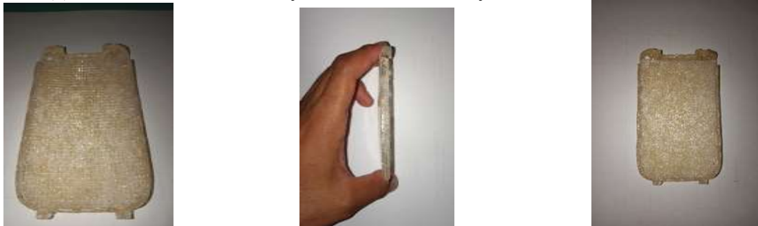
Fig. 2 a, b, c, the real biocomposite of tandanus tectorius cabin lamp cover
