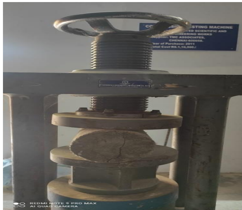
Figure 4. Testing of Split Tensile Strength
