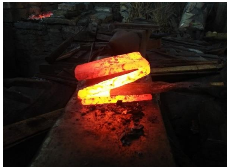
Figure 11. Nickel Insertion Process (First Pumping)
