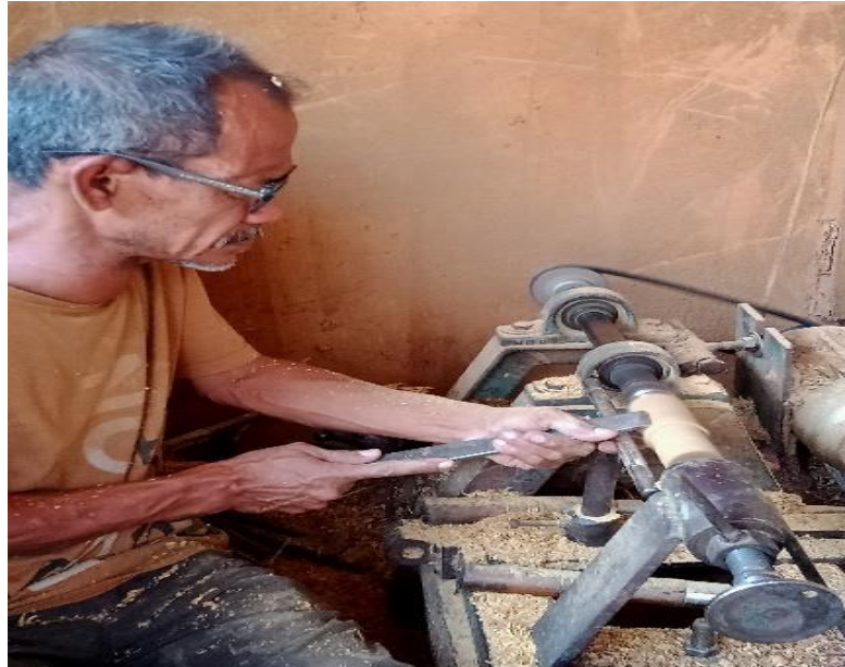
Figure 37. Process of Flattening the Wood with Chisels
