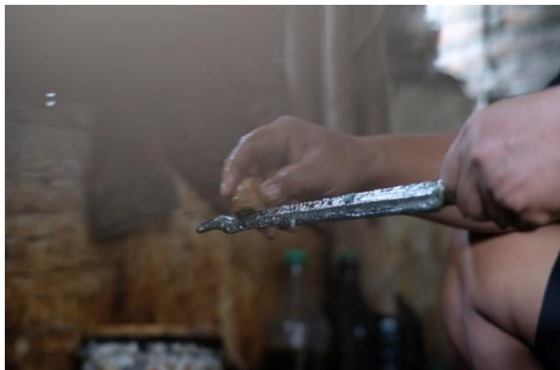
Figure 33. The Process of Cleaning the Blades with Orange Water and Dish Soap
