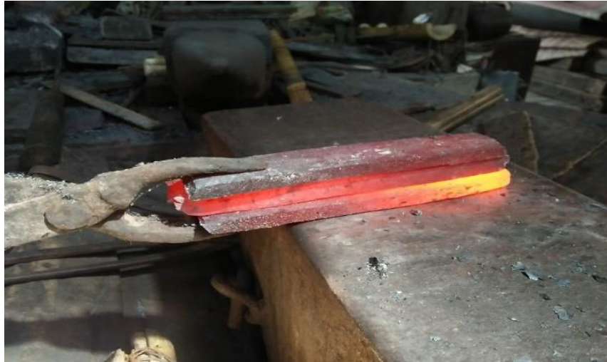
Figure 20. Process of Inserting Steel Into the Saton
