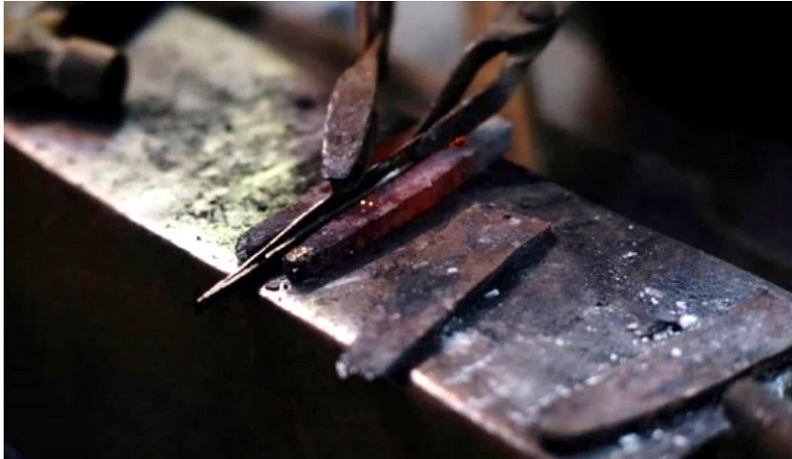
Figure 25. Nickel Insertion in Iron-Steel Uletan
