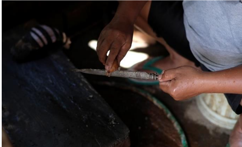
Figure 31. The Process of Cleaning the Blades with Orange Water and Dish Soap
