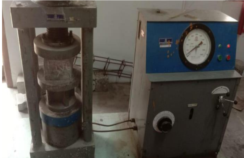
Figure 1. Compressive Strength Test on Cube Specimen
