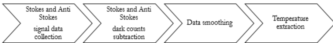
Figure 2. Flow chart of a fibre temperature sensor based on Raman backscattering. Stokes and anti-Stokes signals are collected to be modelled to get the distributed temperature data.
