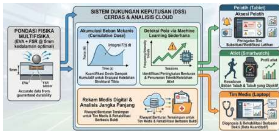
Figure 4. Intelligent Sports Safety System Architecture and Decision Support System (DSS) Integration
