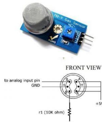
Figure 1. Schematic of MQ-2 Gas Sensor
