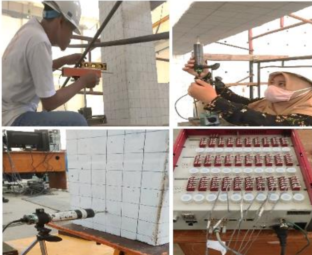
Figure 6. LVDT on Test Pieces and Installation Photos
