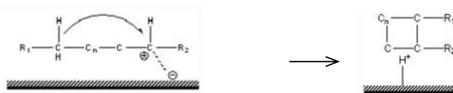
Figure 41. Formation of Saturated Cyclic Compounds (Naphthane) from Alkane Compounds on the Catalyst Surface
