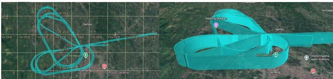
Figure 11. Holding Pattern with Models 1 and 2, with Garmin 1000 data view on Google Earth.
