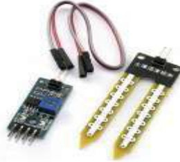
Figure 6. Soil Moisture Sensor Module
