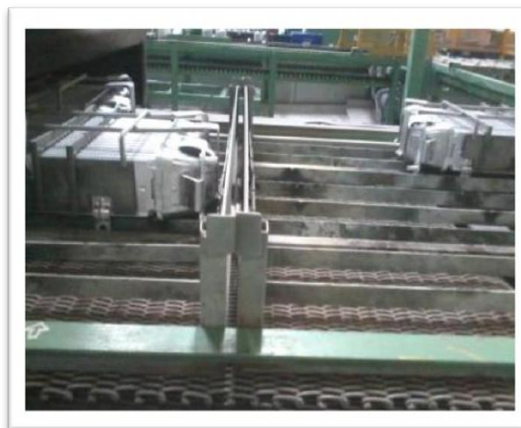
Figure 1. Fixing the spacing between palletes
