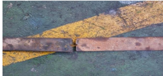
Figure 16. Broken Leaf Springs
