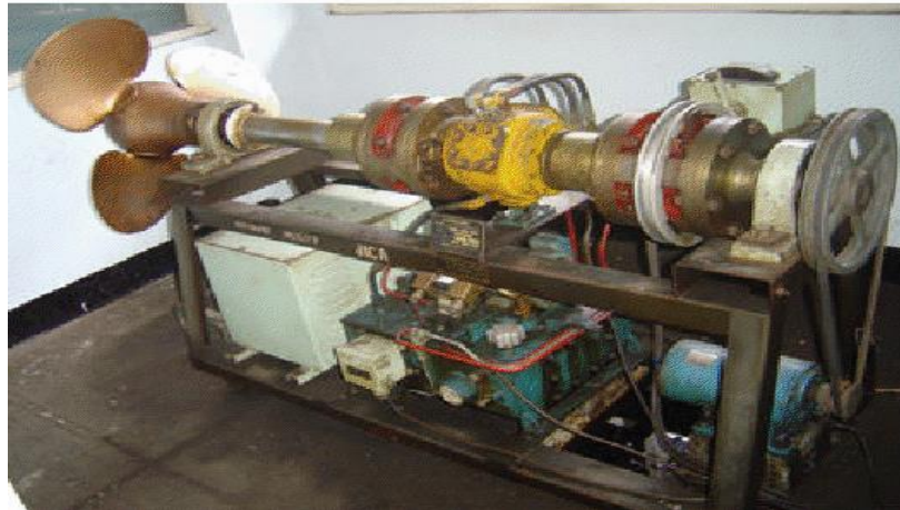
Figure 2. Position of Crankshaft, Gear Box and Connecting Shaft Source: Directorate General of Primary and Secondary Education, Ministry of National Education, 2003
