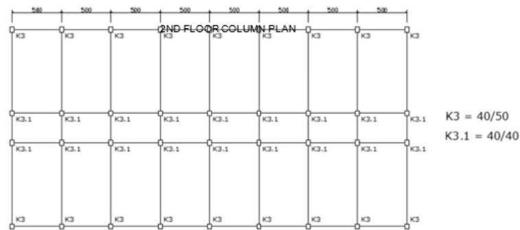
Figure 2. Column Plan of Civil Engineering Department Building
