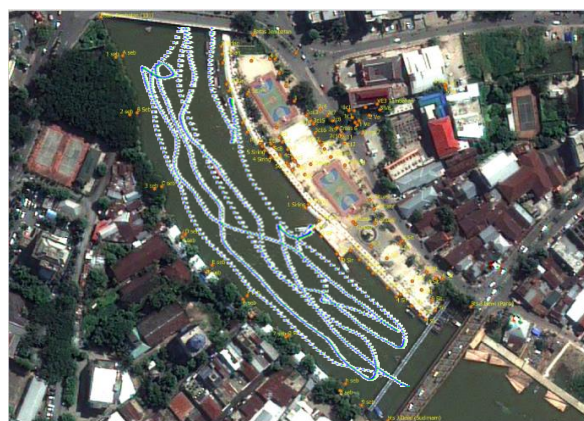
Figure 5. Distribution of Terrestrial and Bathymetry Survey Elevation Points
