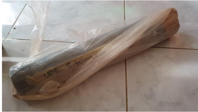
Picture 3. Undisturbed Sample (UDS) at a Depth of 5 Meters
