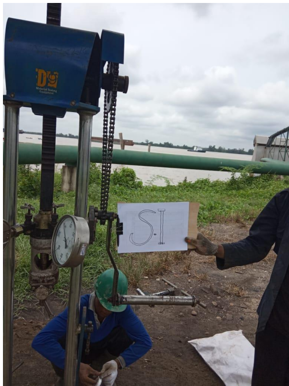
Picture 2. Cone Penetration Test (CPT) Execution at Point 1, River View
